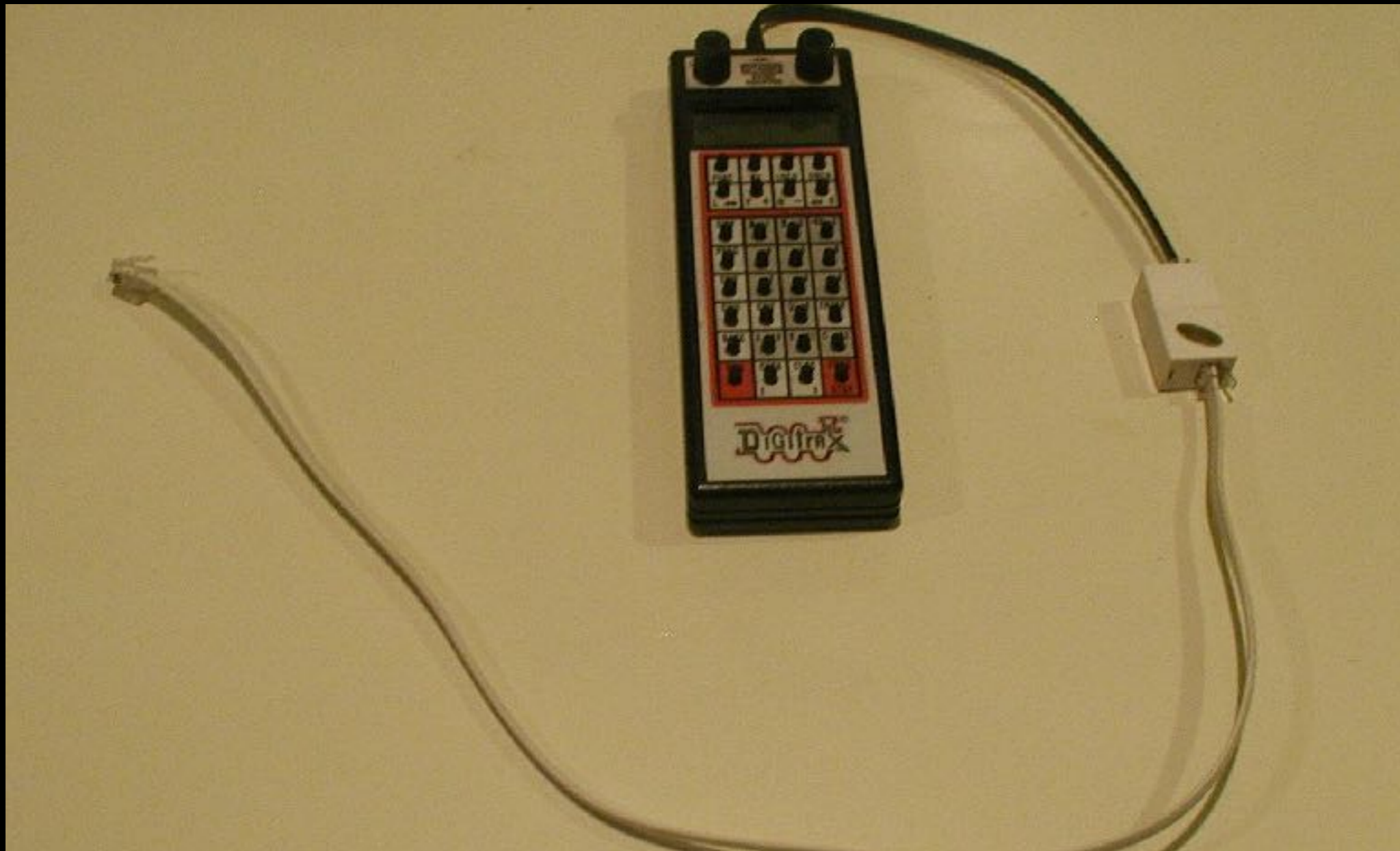
Digitrax Wireless Throttle with Extension for Tethered Operation
